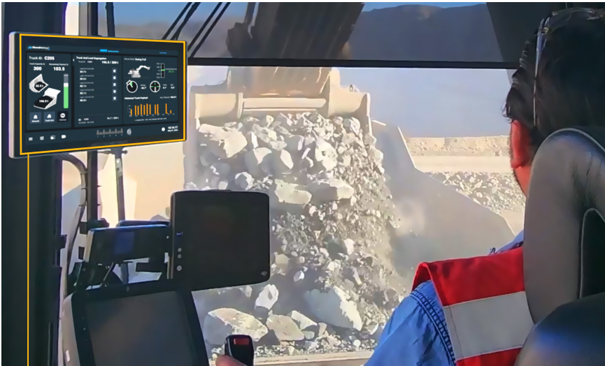
Rugged, easy to use touch-screen operator interface provides real-time payload feedback for bucket and current truckload.
