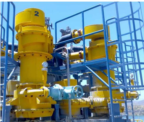
Cavex® DE hydrocyclones with air core boosters, installed at a mine site in Chile
