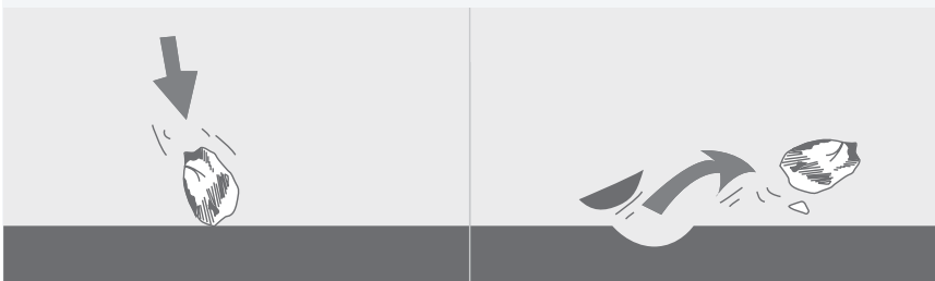
Abrasive particle striking non-elastic metal surface. Conversion of kinetic energy into impact, friction and noise.
