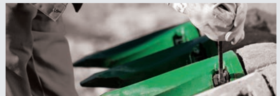
A pry tool is used to lock and unlock the point to the adapter.
