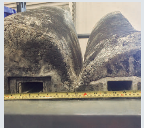
Side by side comparison of Vulco® mill liners with R67 rubber (left) versus R63 rubber (right)
