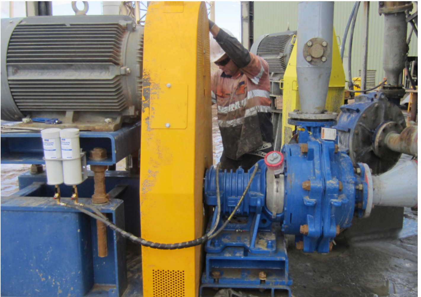
The Warman WBH® pump fitted with Accumin™ automatic grease lubricators
